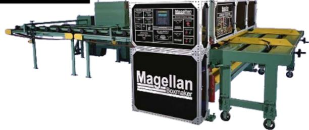
Designed specifically for the manufacture of large format corrugated cartons, the Magellan Boxmaker completes short runs of very large cartons easily.
